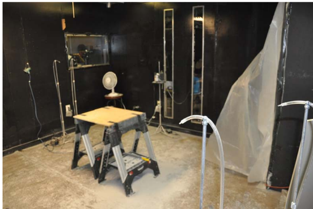
Figure 3. Area air sampling and test chamber configuration.
